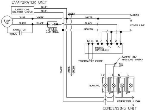
Fig. 2.3 VINO2500-4500SSR Wiring Diagram (DIGITAL CONTROLLER)
